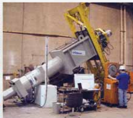
Far left: CTL reoriented its high-capacity fatigue test fixture to a horizontal configuration to accommodate the 8m-long cable specimens
